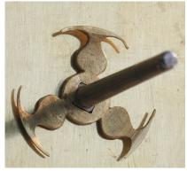
Detail of this rather unusual and nicely cut friction washer on the cannon pinion.
