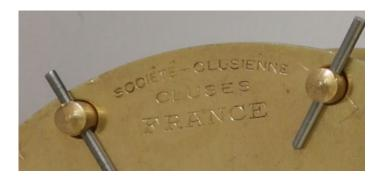
Paris movement from an *ebauche* by the Société Clusienne (Cluses, France). Half-rollers escapement and steel suspension from the patents by Achille Brocot, countwheel strike on the hours and half-hours on a silvered bell, autonomy of two weeks.
