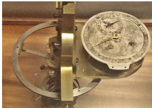
Fig. 1. Pierre Le Roy's marine chronometer, 1766
